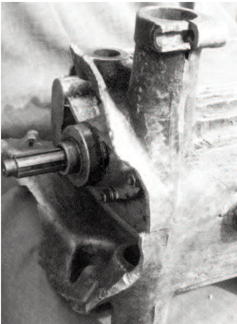
E.N.V. C-type box showing cross-tube mounting. Bell housing was trashed when the clutch exploded during racing! (Barry Foster)
