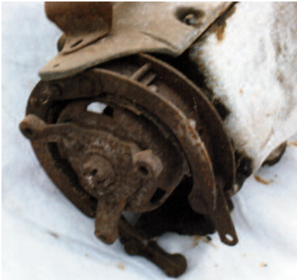
Early M-type showing bracket for fixing transmission handbrake (Barry Foster)
