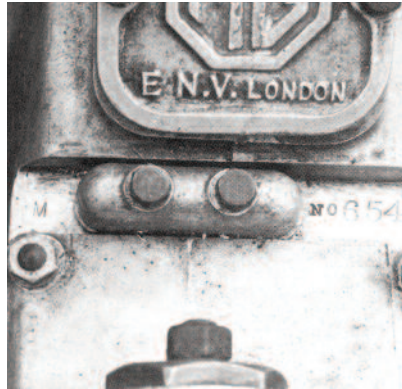
E.N.V gearbox no. 654 with 'M' for modified input shaft (Barry Foster)
