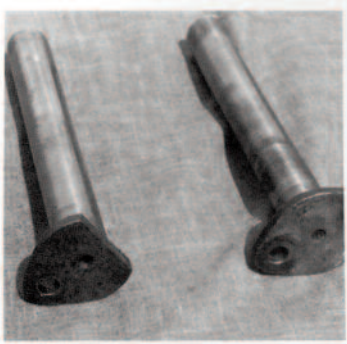
E.N.V reverse gear shafts. Close ratio shaft has single fixing hole (Barry Foster)
