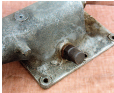
E.N.V reverse gear - gate spring housing (Barry Foster)
