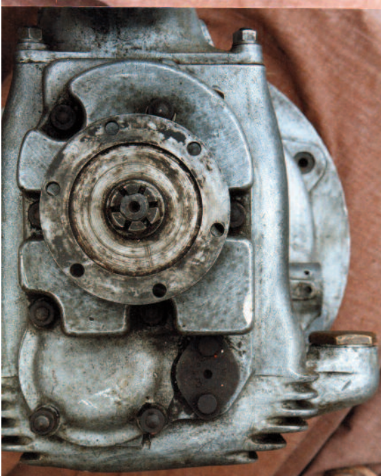
E.N.V. rear end showing position of reverse gear shaft, standard gear ratios. (Barry Foster)
